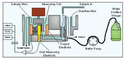
The sample stream runs down through the lower block, where it mixes with vinegar (and potassium iodide where total chlorine is being analyzed), and then flows upward through the measuring cell. Within the cell, the vinegar provides pH buffering to a value of 4.0, and aids in keeping the cell clean.
